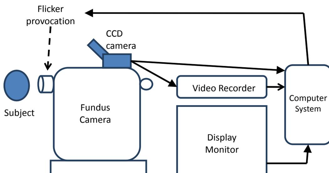
Figure 3.1 Diagrammatic representation of the dynamic retinal vessel analyser set up
