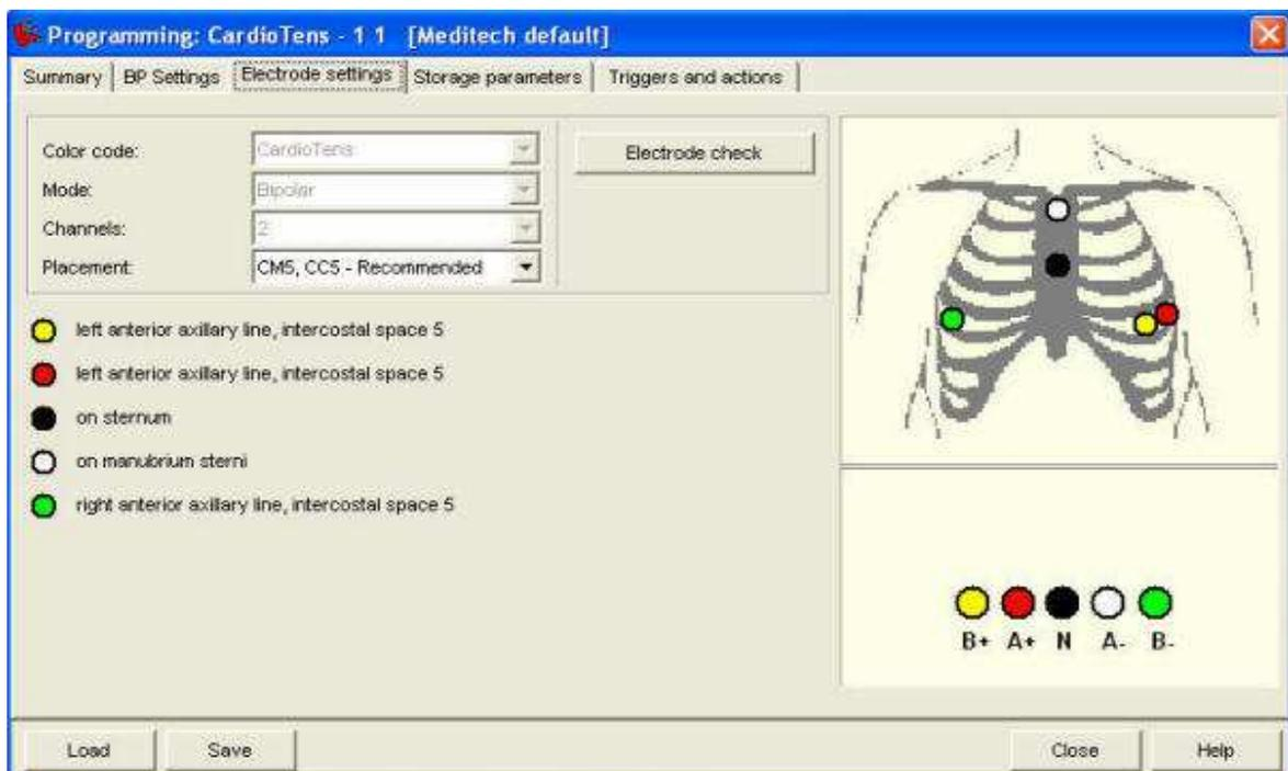
Figure 3.9 Diagrammatic representation of the electrode positioning for 24 hour ECG recording with the Cardiotens-01 device
